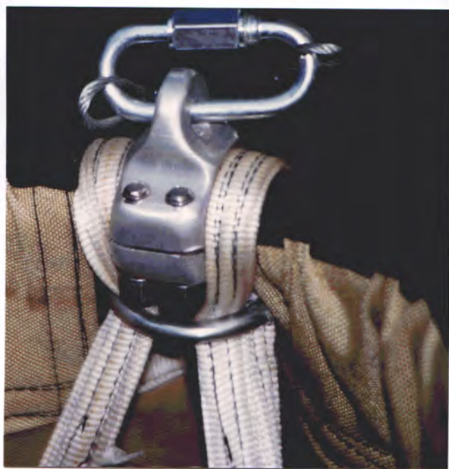
Figures 3 and 4: A drawing and photo of the vertical tube end fitting. The eye on top of the fitting is used as an attachment point for lifting the entire basket assembly. My drawing shows an optional countersunk clamping screw mount. John left his screw heads exposed.
