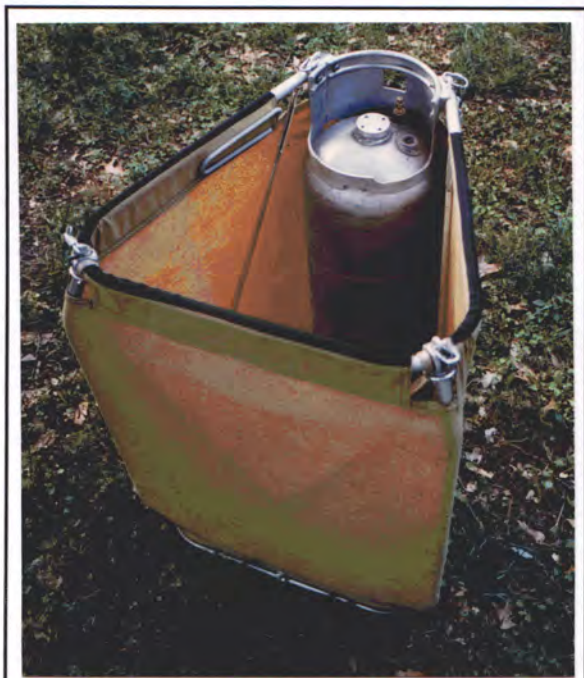
Figure 1: John Burk's basket is constructed of aluminum and fabric. It weighs 44 pounds. The tank is permanently mounted as one corner of the basket structure.
